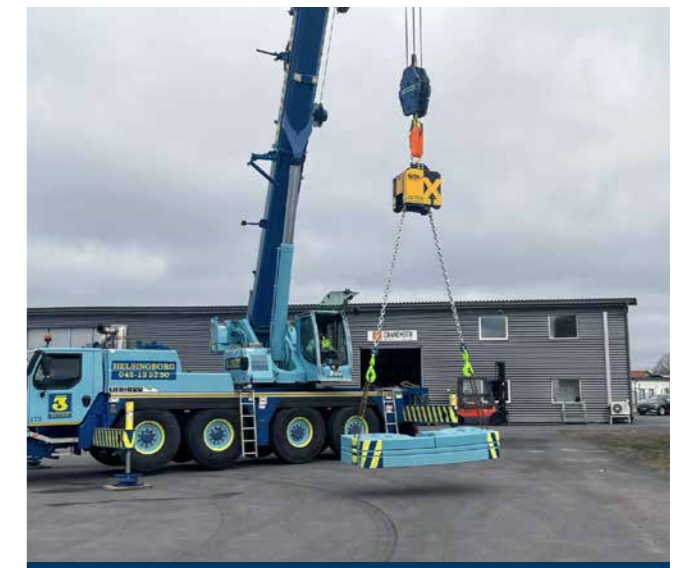
Levo load balancer equalising crane counter weight
